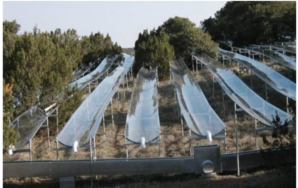
Precipitation manipulation experiment, Sevillita LTER, New Mexico. The troughs exist to limit precipitation on plants, simulating drought conditions. William T. Pockman, University of New Mexico https://www.fs.fed.us/research
