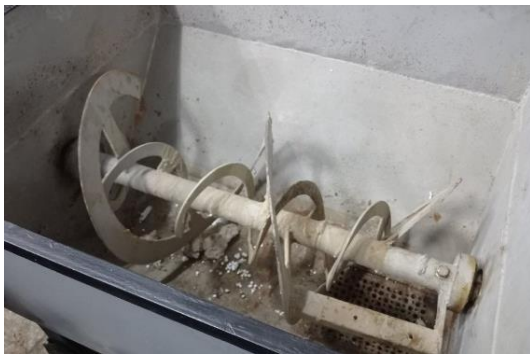
Figure 10 – Mixer for preparing construction mix
