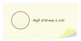
When the permissible deviation in size is very small, we say it is a tight tolerance (or a close tolerance). A large permissible deviation is a loose tolerance. For example:
